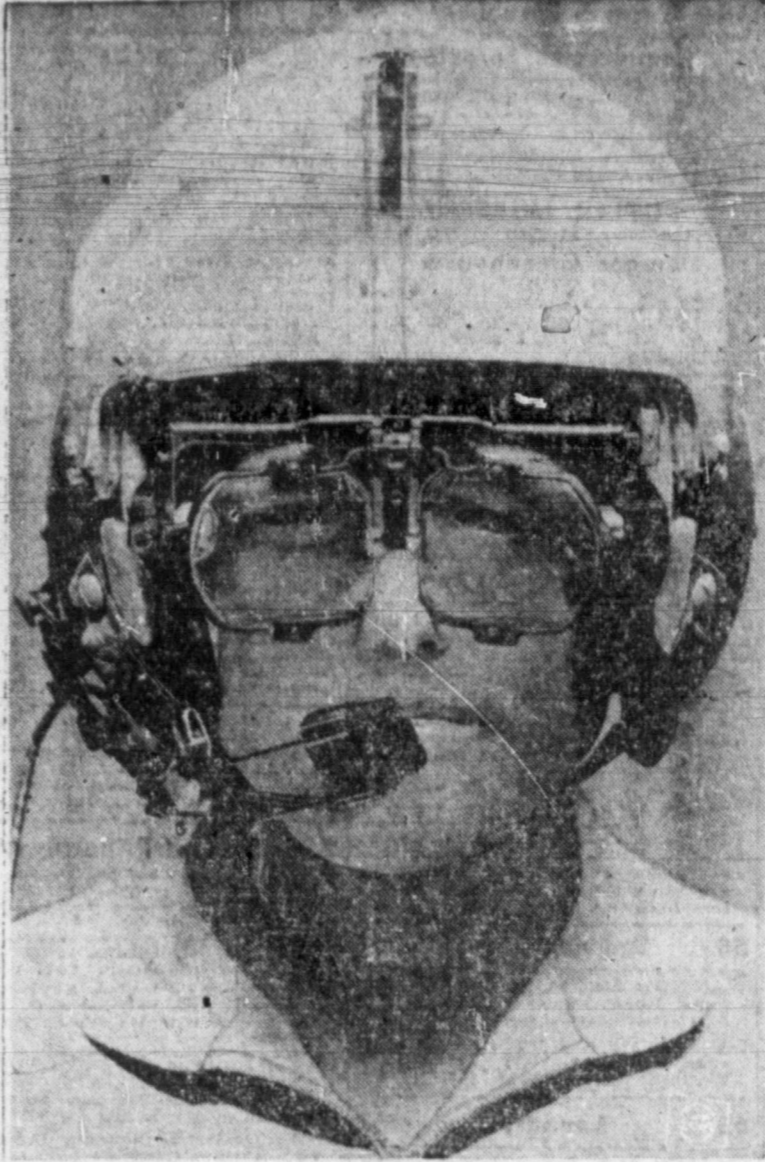
FOUR EYES—Eye glasses developed by the Bell Helicopter Co., permit wearer to see things as they are but with a superimposed second scene over the real view, to produce a controlled double exposure similar to a motion picture title appearing over a movie background. This is accomplished by projecting an image onto the surface of the lenses by optical or electronic methods. Device enables pilot to watch his instruments as he scans flight path.
