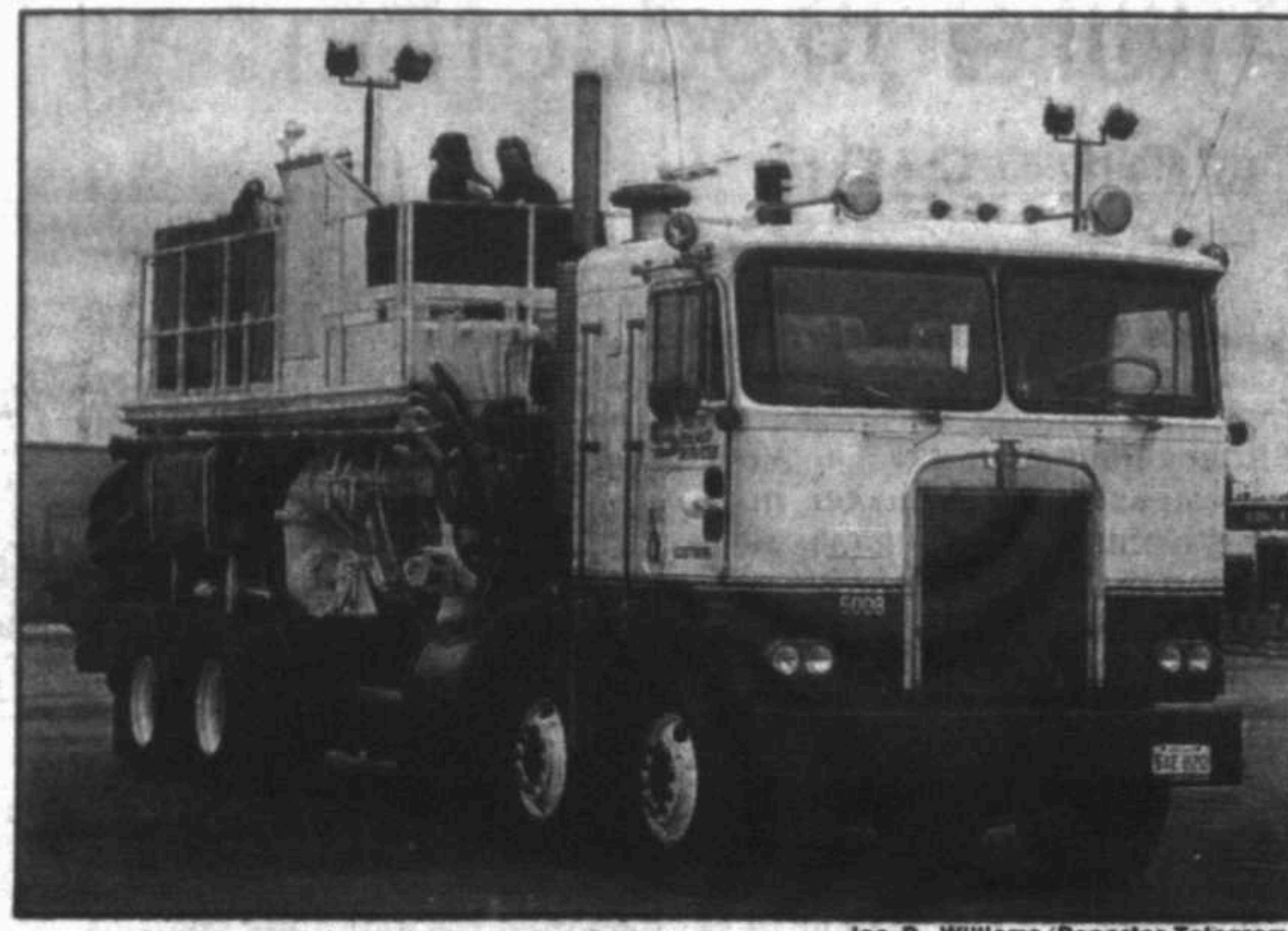
This on-the-fly blender, which mixes and pumps stimulation chemicals downhole, is just one new development the stimulation industry has seen over the past few years.
