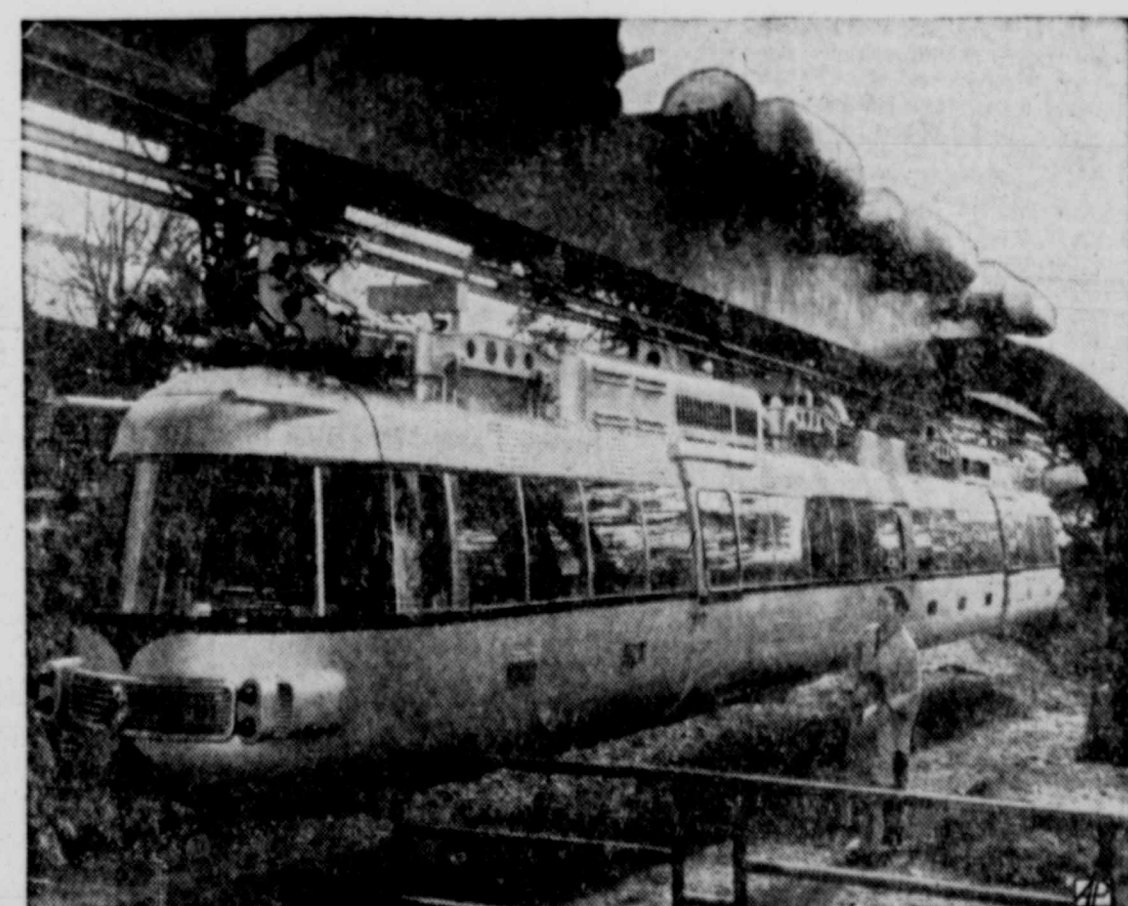
OVERHEAD RAILROAD — Experimental model of Japan's first monorail train is exhibited in Tokyo park. The two-coach electric train, an effort to unsnarl Tokyo's mounting traffic problem, can carry 62 people along a single track suspended 15 feet above the ground.
