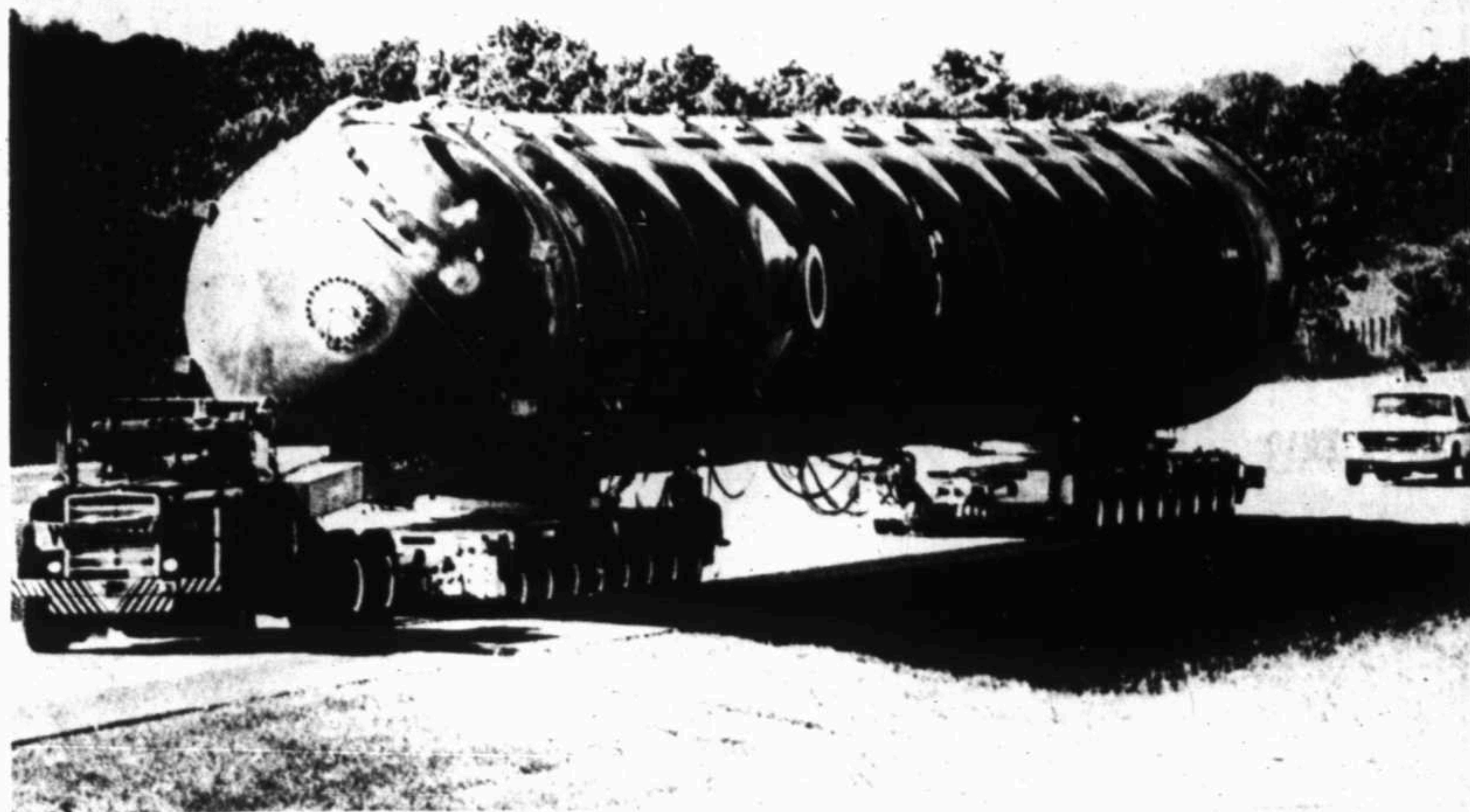
This high petrochemical vessel 174 feet long and weighing 360 tons made its way down Houston streets to the Houston Ship Channel for a barge ride
