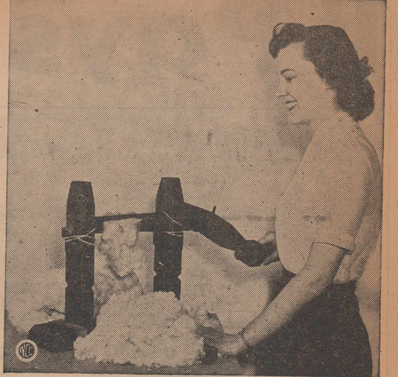
It's a cotton gin all right. It will be shown at the Mid-South Gin Machinery and Supply Exhibit in Memphis, March 10-12. This Churrka gin is said to pre-date Eli Whitney's invention by several centuries, having been used by the ancient India Hindus as early as 3,000 years ago. The young lady seems to have no trouble operating it—far cry from the complex cotton gin of today!
