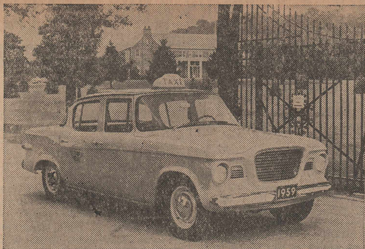
The new Studebaker Econ-O-Miler taxicab is mounted on a 113-inch wheelbase and is powered by the new, economical six-cylinder engine developed by Studebaker engineers. It has an increased compression ratio and operates efficiently on regular gasoline.
