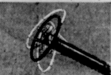
Tilt-telescopic steering wheel moves up or down, in or out, can be added to any model
