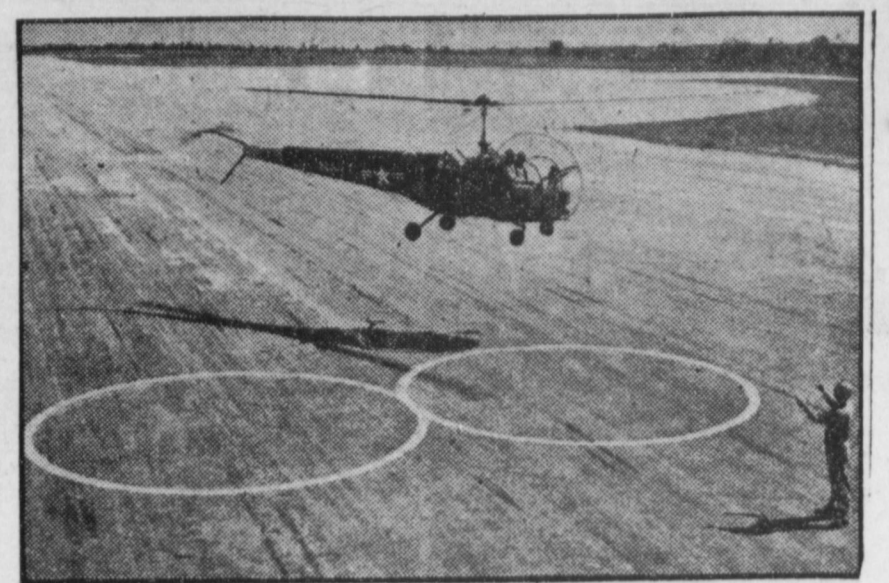
FIGURE FLYING—The Navy's new helicopter training program at Pensacola Air Station, Fla., includes this figure eight flying exercise. At a height of 10 feet, the craft is maneuvered over the numeral painted on the runway. The new helicopter instruction was started in response to the growing proof of the value of the planes in Korea.
