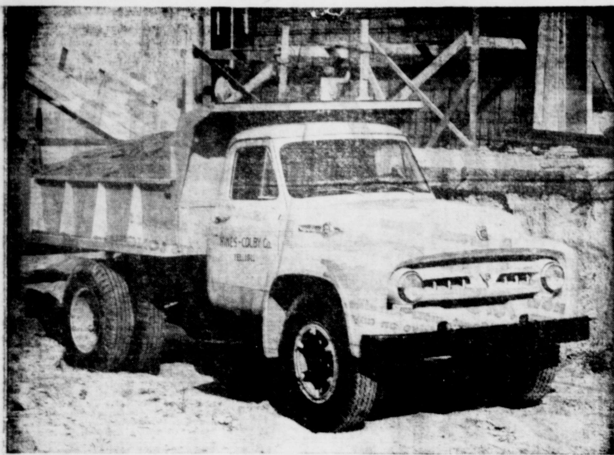
The F-900 is the new heavyweight leader of the 1953 Ford truck line—the biggest truck ever built by Ford. Powered by a Cargo King overhead valve V-8 high compression, low friction engine, it has a front axle capacity rating of 8,000 pounds and a rear axle rating of 21,000 pounds. Its wide range of wheel-bases makes the F-900 suitable for all types of extra heavy-duty on or off-the-road work. Its maximum GVW is 27,000 pounds and maximum GCW 55,000 pounds.
