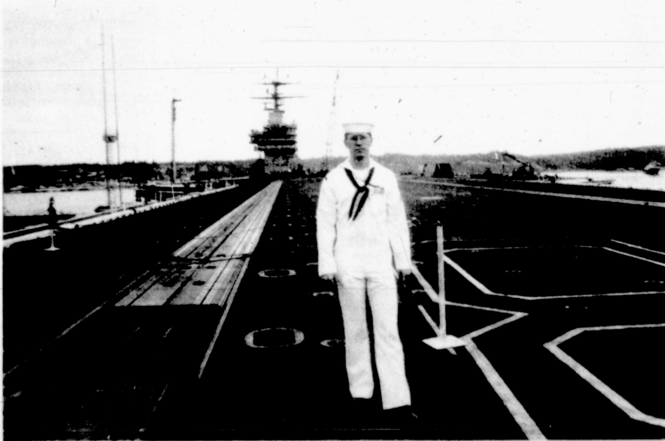
Seaman Kelly Hendrick stands beside one of the ship's four Type C Mark 13 Mod 1 catapults, capable of propelling the heaviest carrier aircraft from the flight deck at speeds in excess of 170 miles per hour, reached in less than three seconds after a standing start.
