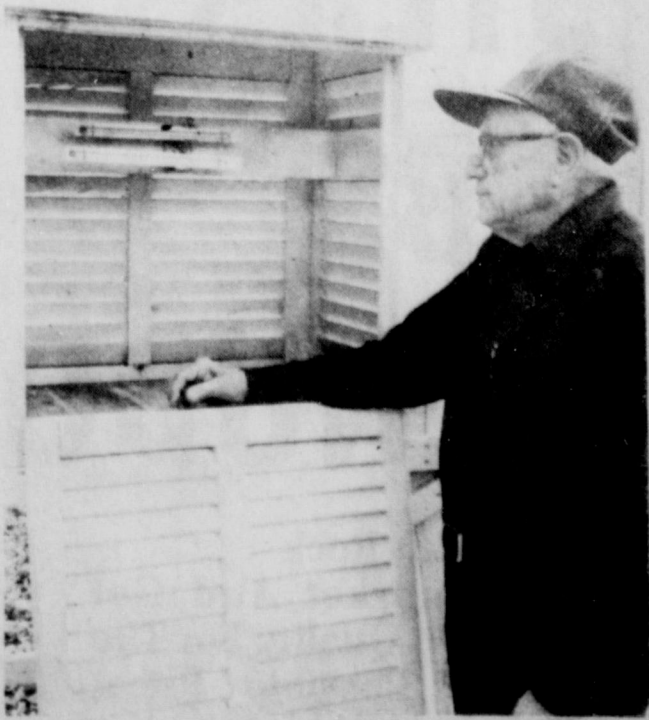
FRANK HILL, Tahoka's weather reporter, displays the louvered box used to house the two unique thermometers used in his daily records.
