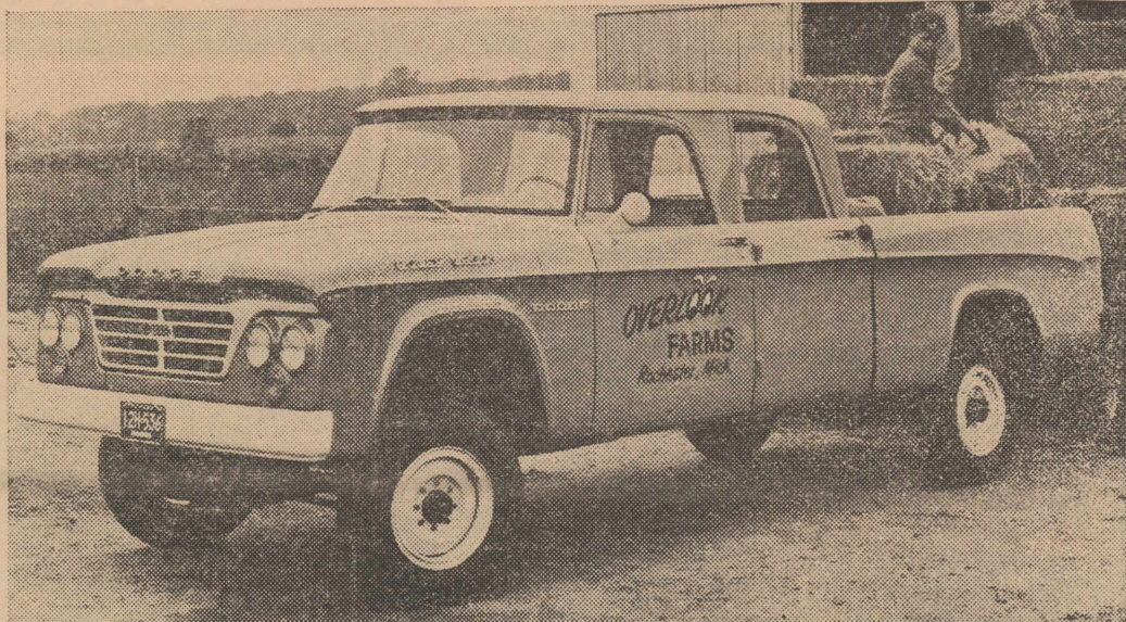
VERSATILE TRUCK —Capable of carrying six passengers and a payload of more than 2,000 pounds, this Dodge W-200 pick-up truck with Crew Cab and four-wheel drive is especially useful on the farm, ranch, construction site or utility installation. Shown here with a 6½-foot Sweptline pick-up body, the W-200 has a 146-inch wheelbase. The standard engine is a 140-horsepower, 225-cubic-inch Slant Six.
