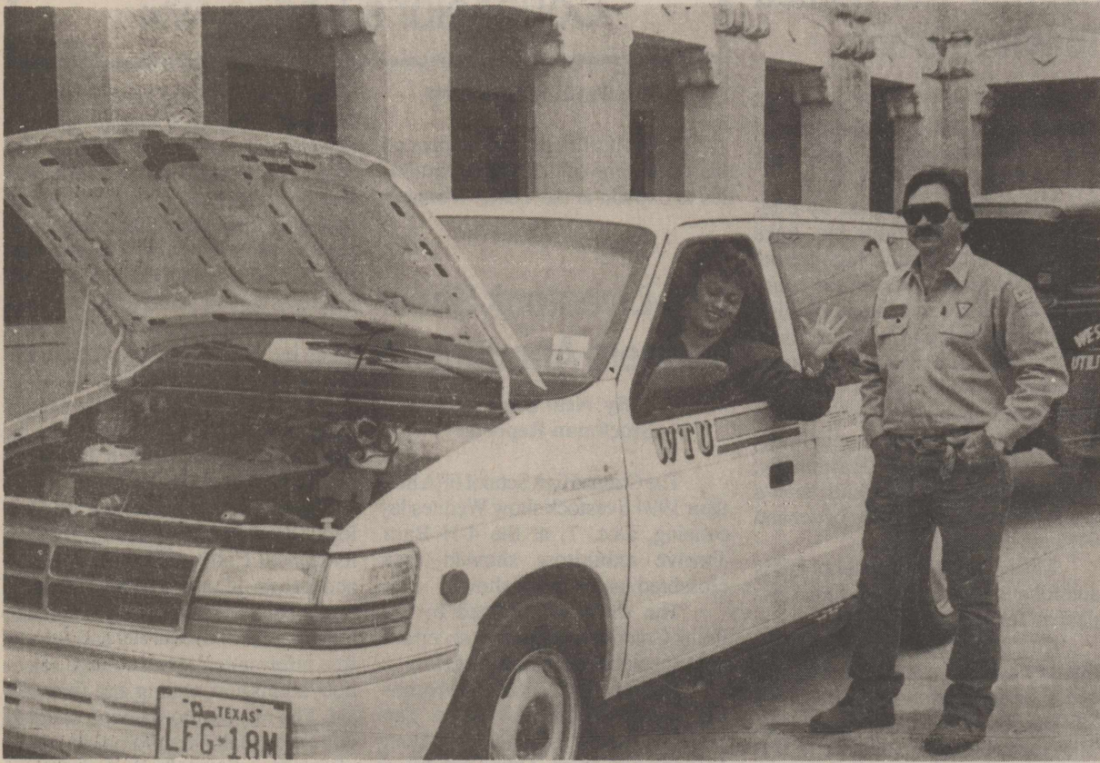
WTU ELECTRIC VAN - Debra Tambunga and Armando Arredondo check out a new electric 1994 Dodge Caravan at last Wednesday's WTU open house. The electric vehicle gets 60-80 miles to the charge, charges in 8 hours, runs on 30 - 6 volt batteries and costs $125,000. photo by Neal Ulmer
