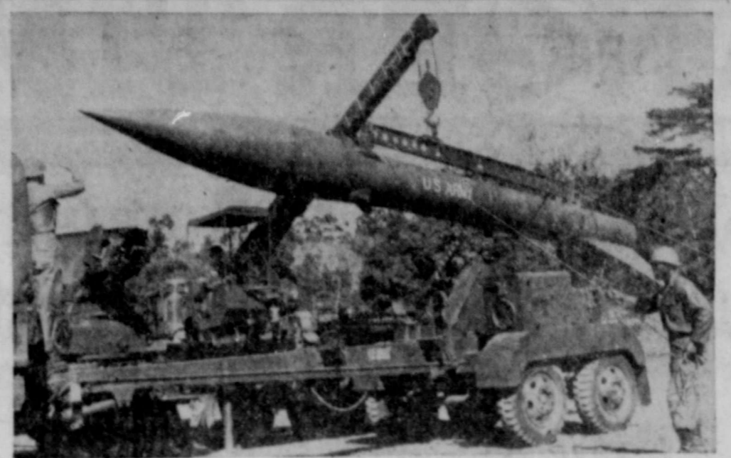
CONNING IT HOME—U.S. soldiers at home and abroad for several years have appreciated the simplicity of operation of the needle-pointed Honest John, a free-flight artillery rocket shown being cradled into a truck-mounted launcher by 25th Division troops in Hawaii.
