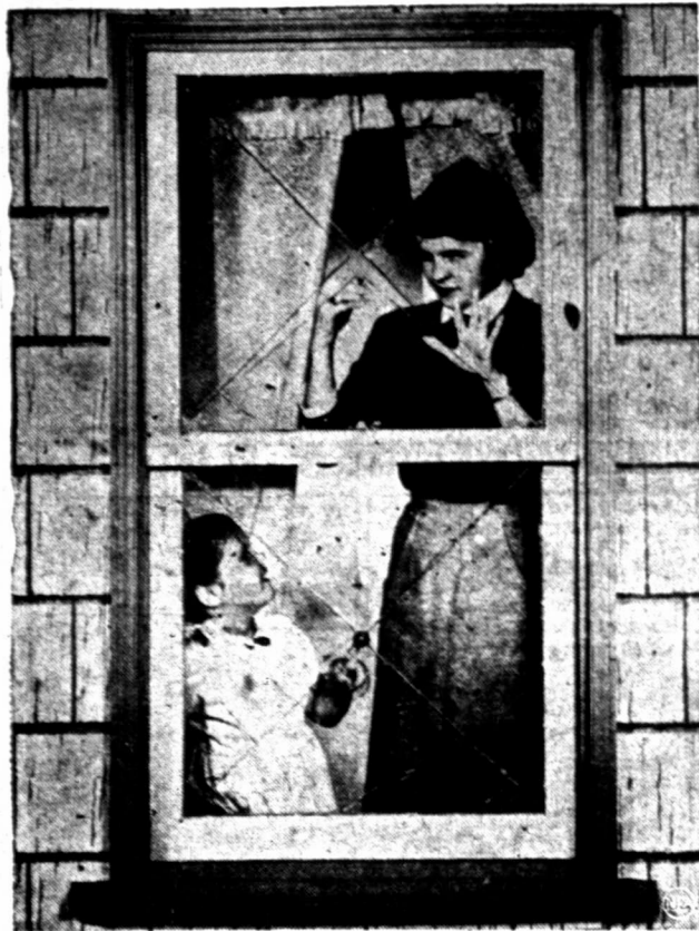
WINDOWS WITH A BUILT-IN "CRASH" —This special window, designed to reduce hazards of flying glass during a bomb attack, was developed by the Pittsburgh (Pa.) Plate Glass Co. When hit by blast pressure, the window's four triangular sections, sealed together and hinged to the frame by a glass-plastic laminate, automatically give way. Top window has broken apart, minus any flying glass fragments. Bottom window has been repaired after crash by use of a fastening bolt at center. Adhesive tape, putty or chewing gum will serve same purpose.
