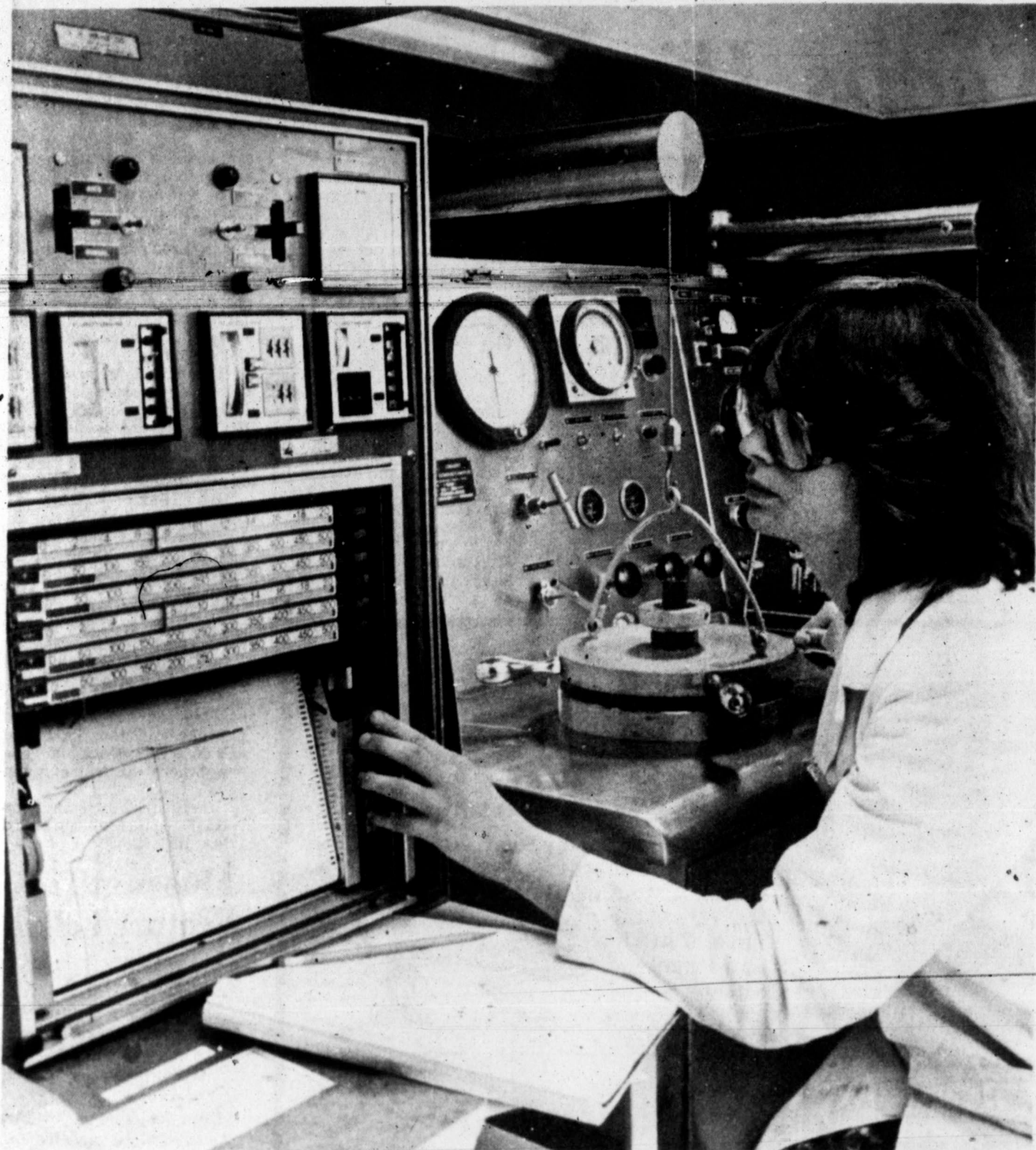
HOW IT IS BELOW —Want to know what it's like 16,000 feet down in a wildcat well in Wyoming? Halliburton technician Jody Allen can recreate the pressures and temperatures encountered in such a well at Halliburton Services' Research Center.
