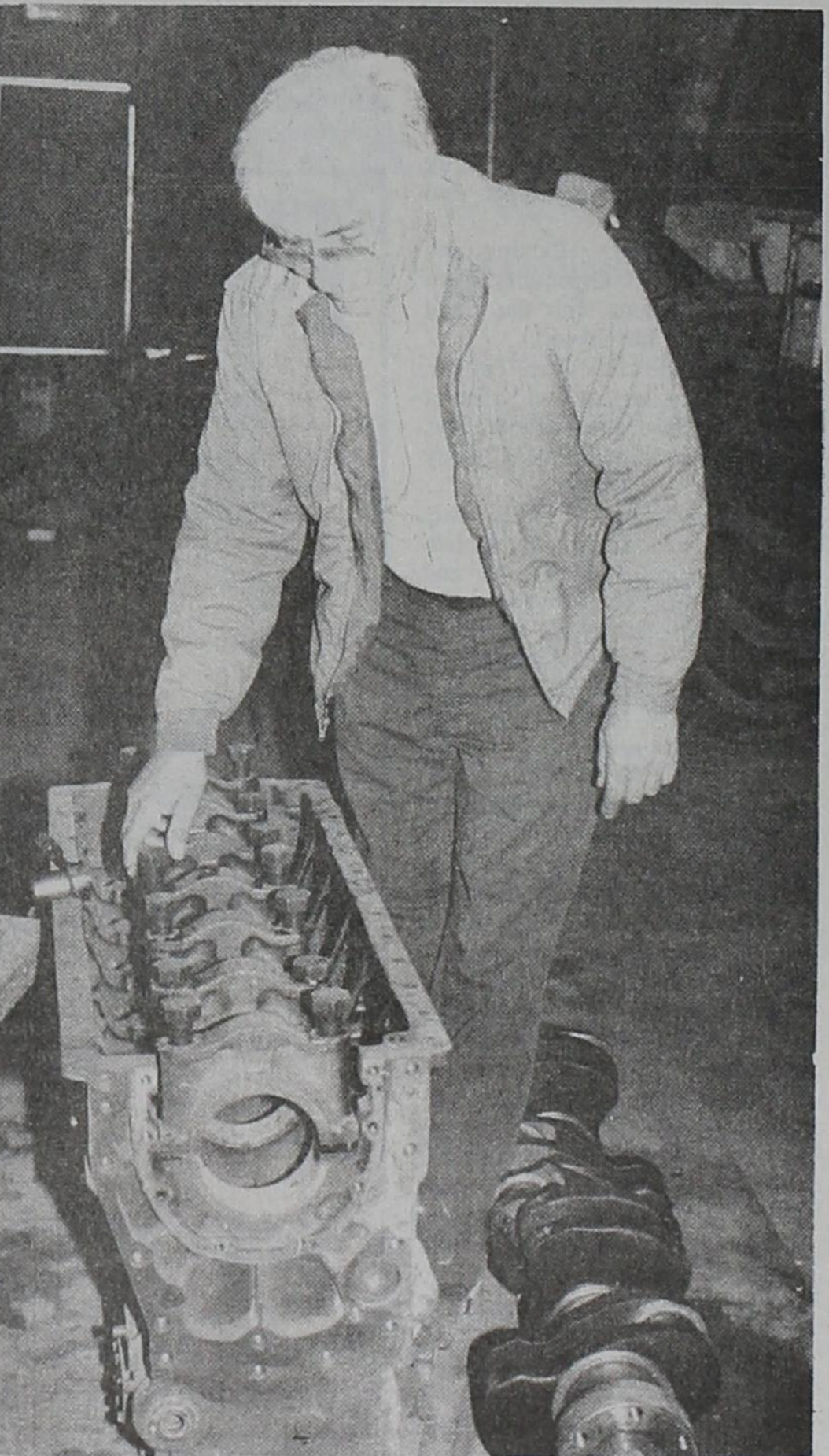
RALPH SALINAS , foreman of the Dimmitt Public Works Dept., works on a short block for one of the giant land-movers in use at the city landfill. Salinas was honored by the city recently for his efforts at repairs that have saved the city thousands of dollars.
