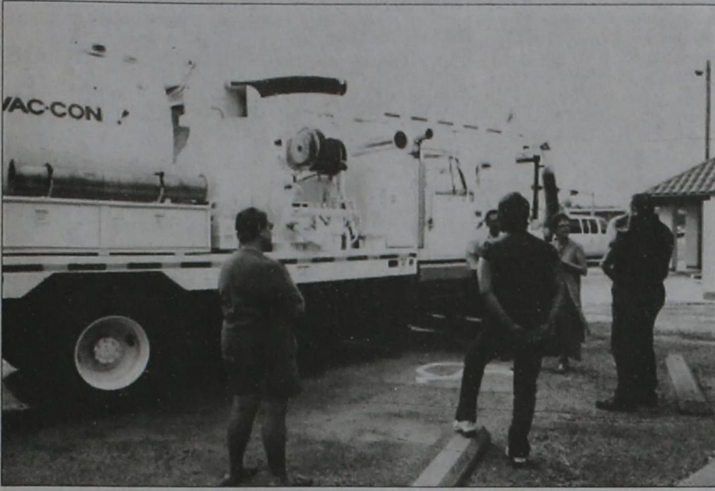
Carolyn Tobias (from left), City Councilman Dick Odom, Mayor Thressa Harp and City Manager Arbie Taylor look over the Vac-Con truck recently purchased by the City of Post. According to Taylor, primarily the water and sewer departments will use the machine. Clogged sewer lines can be unclogged and cleaned using the "jet-rodder" attachment at the front of the vehicle. It can also be used to vacuum manholes and storm sewer inlets to remove debris. Other uses include pumping water out of holes during water main breaks and "hydro-excavation" using high-pressure water spray with the vacuum function to remove dirt from excavations where there is the potential of damage to other utilities using standard backhoe excavating techniques. Hydro-excavation can also help locate the other utilities, such as gas, electric, and phone lines without digging with a backhoe. Photo by Rosa Latimer
