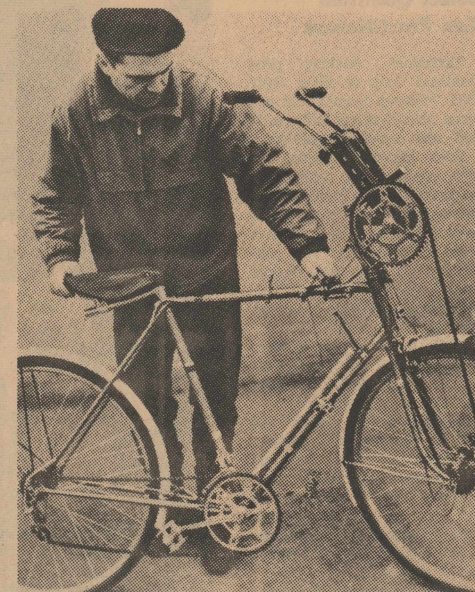
FRONT-WHEEL DRIVE is the new departure in bicycles in the Soviet Union. Leonid Dutov, researcher at Gorky University at Kharkov in the Ukraine, developed the front-wheel mechanism operated by the hand movements that enables rider to climb steep inclines and cover rugged terrain with ease. A Kharkov plant is considering producing the bike for public use.
