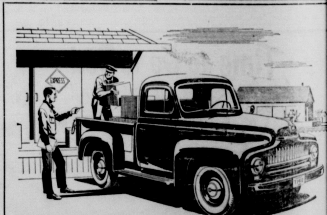
Model L-110, 115-inch wheelbase, 6½-foot pickup body, 4,200 lbs. GVW. Pickups in the L-110, L-120 and L-130 Series include 115, 127 and 134-inch wheelbases, 6½, 8 and 9-ft. bodies, GVW's to 8,600 lbs.
