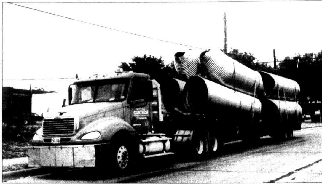
TOO TALL – This semi-tractor trailer carrying metal culverts tried to pass under the railroad track bridge over S. Hwy. 163 last week. Unfortunately for the driver, his load was too tall and hit the bridge, bending the culverts back.
