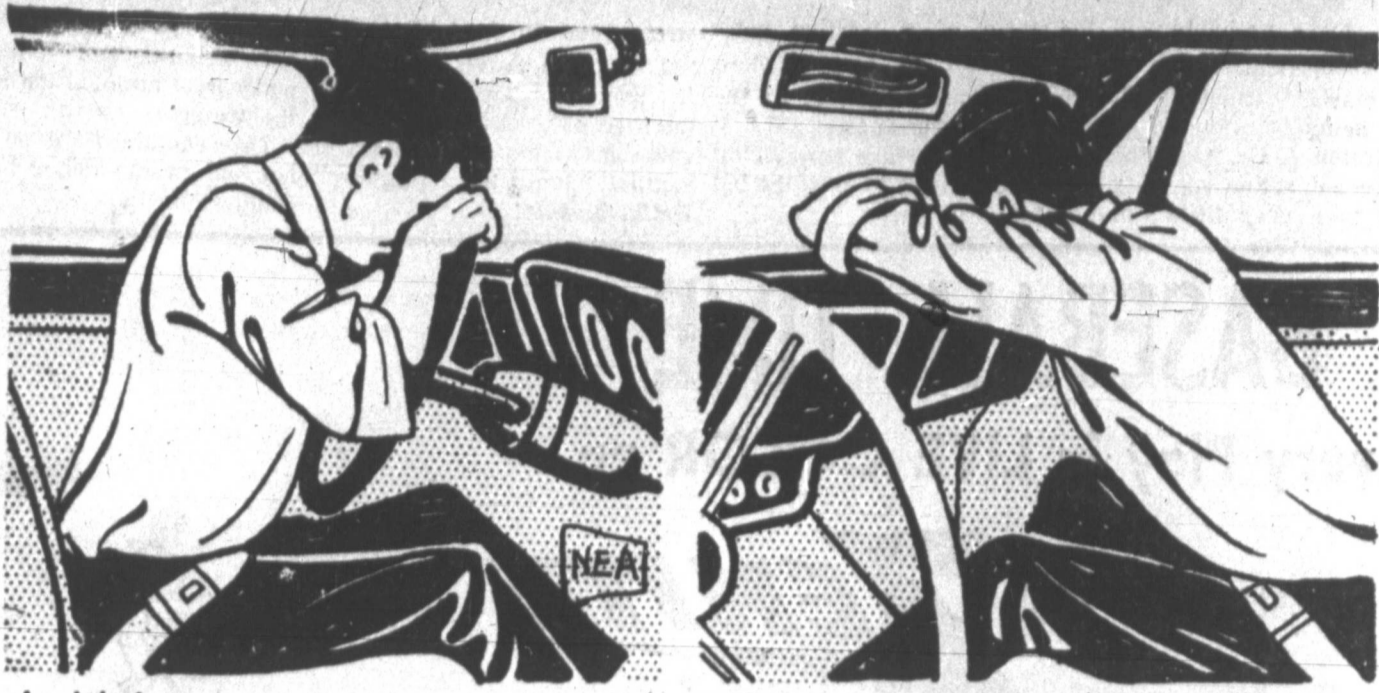
Lap-belted occupants can reduce severity of an impending auto crash by more than 80 per cent if they assume the positions above. If a crash is anticipated, the driver should have both hands on the upper rim of the steering wheel with his elbows out. He can maintain control of the car until the very last moment, when he lowers his head to rest on the back of his hands. A passenger, right, should lean forward as far as possible, place his forearms on the top of the instrument panel and cradle his head above the level of the panel. Findings are results of experiments conducted at General Motors proving ground.
