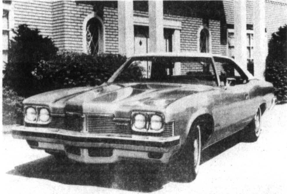
1973 CATALINA — The popular Catalina has all-new front end sheet metal with the grille extending the full width of the front providing a strong horizontal theme. The Catalina has a front bumper system which meets the requirements of the Federal bumper standards by being completely self-storing in a five-mile-per-hour barrier test. Bumper guards and rub strips are available.
