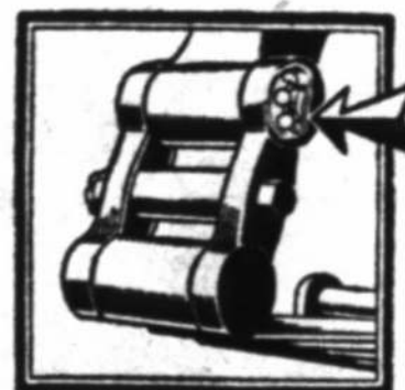
Literally beating the chassis friction-free on 173 balls of polished steel, Studebaker's exclusive ball bearing spring shackle permit unhampered action of Studebaker's pilot springs and hydraulic shock absorbers. Lubricated sufficient for more than 20,000 miles is needed in each axle. They will never bind, nor squeak, nor rattle. And because of all metal construction, there is no deterioration.
