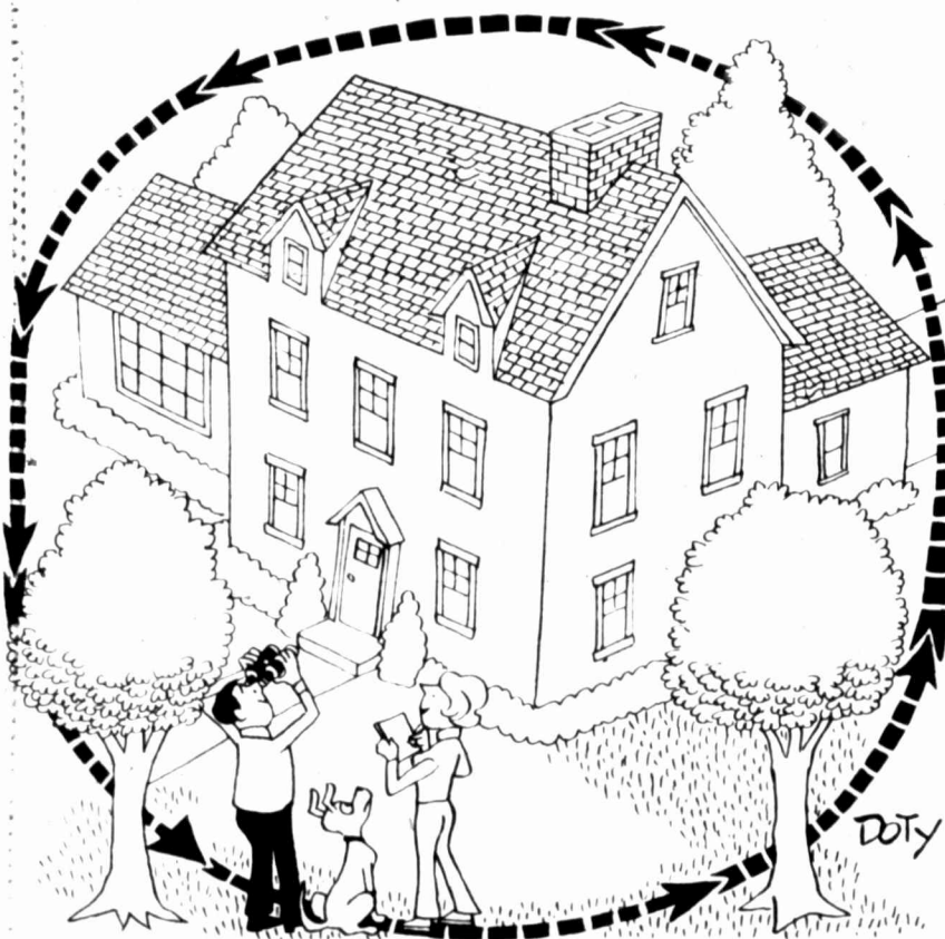
A good way to determine the condition of the roof is to take a walk around the house with a pair of field glasses. Look for cracked, curled or missing shingles, says the Asphalt Roofing Manufacturers Association. They are signs that the roof may need to be replaced.
