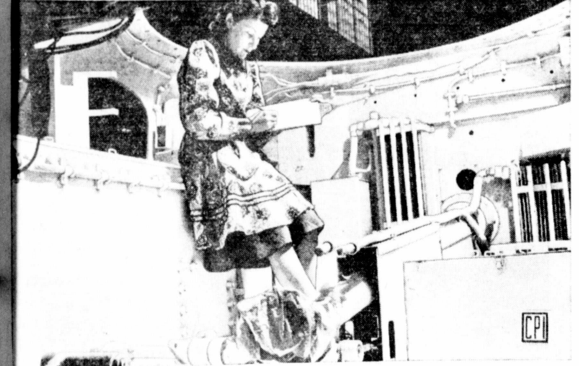
A trick of the camera gives the interior of this Ram tank a cavernous appearance. By the time all armaments and fittings are installed there will be just enough elbow room to permit the crew to operate efficiently. Rotary turret on a Ram tank gives gunner a maximum range. The girl is checking installation of equipment.
