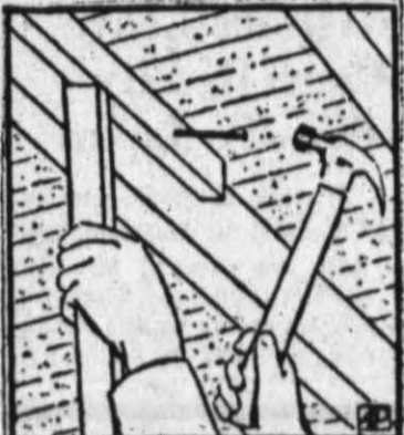
SQUEAKS at several points can be combatted by nailing a hardwood strip to a joist with screws up into the floor.
