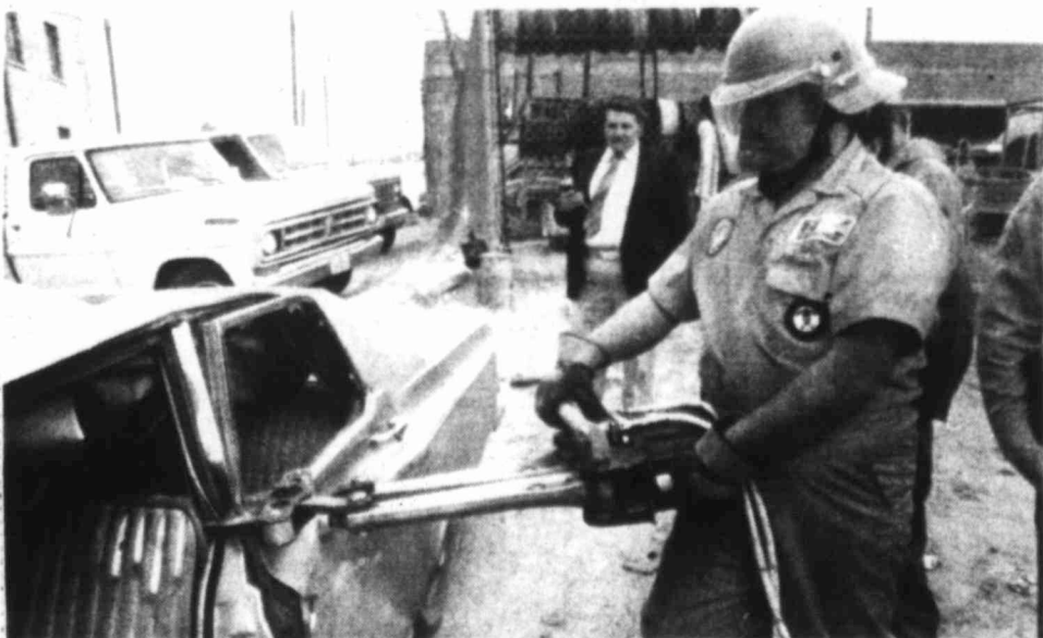
... cut columns away and push the dash up
