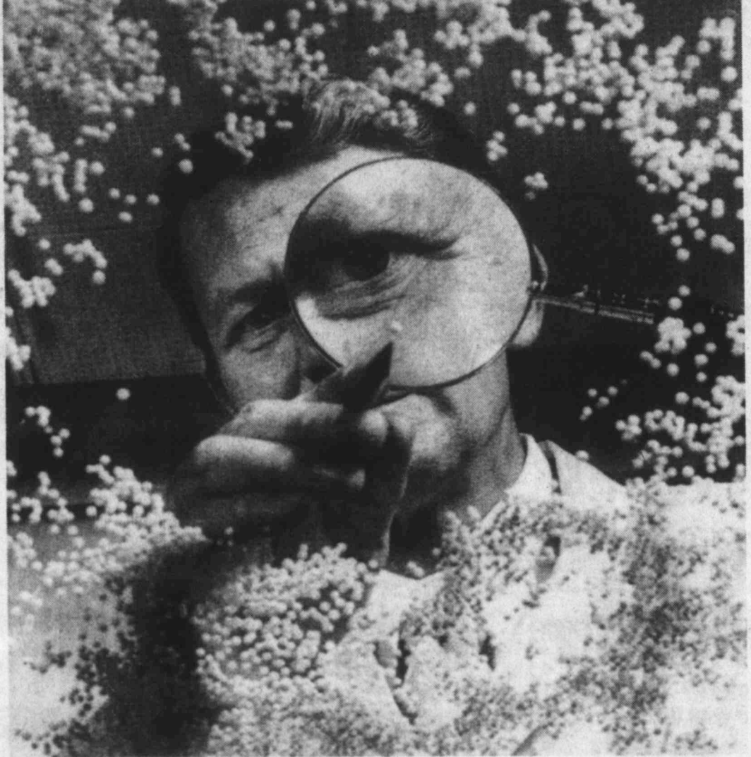
DRAWING A BEAD — A porous silica bead which can be used in proposed auto emission control systems, is examined under a magnifying glass. The long-life beads, developed by PPG Industries at their Harnarville, Pa., glass research center, improve efficiency of industrial chemical and
