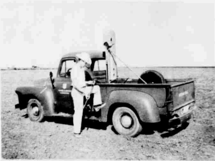
Examination Of The Soils A hydraulic core sampling machine mounted on a pickup truck was used to examine many of the soils in Lamb County.
