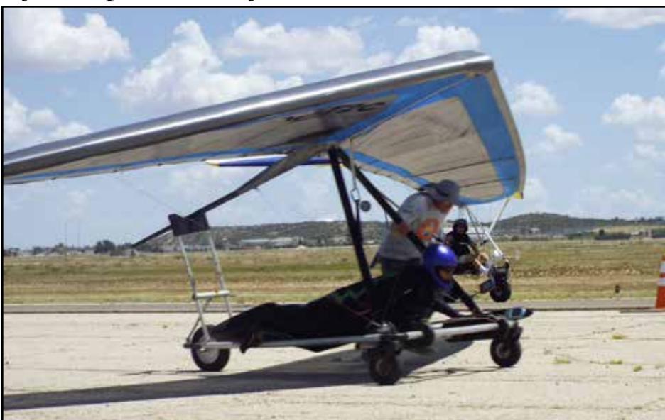
HERALD photo/Roger Cline A pilot prepares to launch from a tow dolly. Gliders are towed behind an ultralight tow plane to a height of about 2,000 feet.
