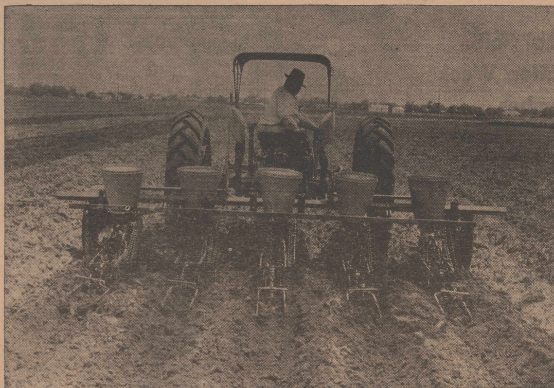
This specially designed 5-row planter will put down cotton in 28-inch rows in the same space as four standard rows. This is to prevent rankness in cotton on irrigated land and encourage heavier fruiting.
