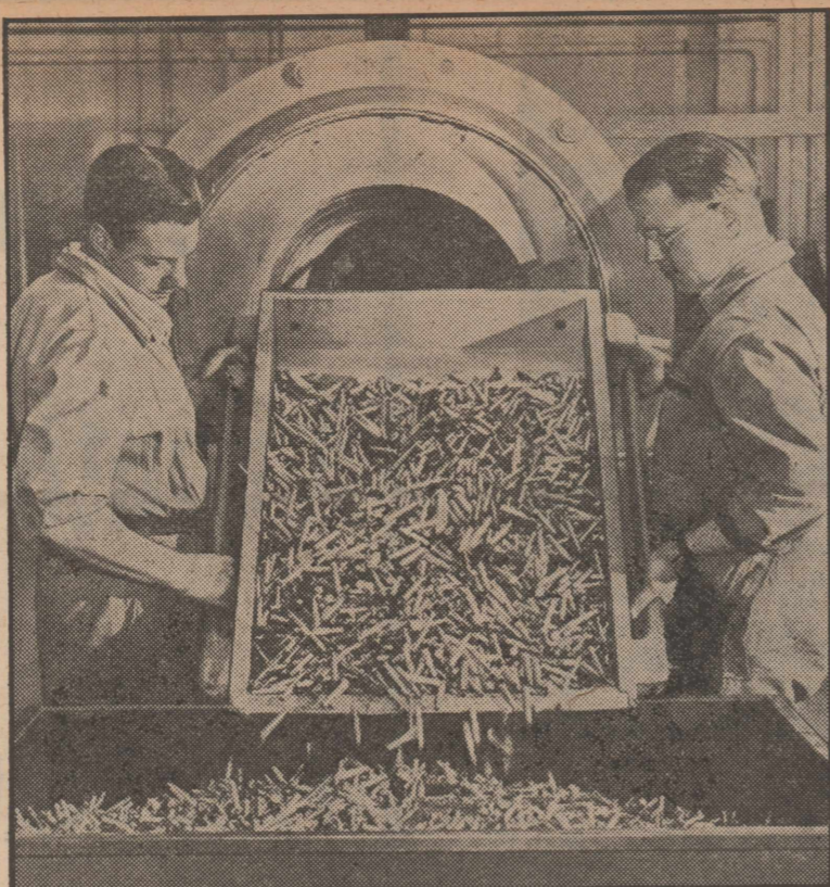
THE OLD (DEADLY) SHELL GAME —A Dutch factory, the Artillerie-Inrichtingen (artillery works), established in Amsterdam, The Netherlands, in the 17th century, is today producing arms and ammunition for the 20th century armies and navies of the North Atlantic Treaty Organization. Two of the company's employes, above, unload .303 caliber shells into a final processing hopper.
