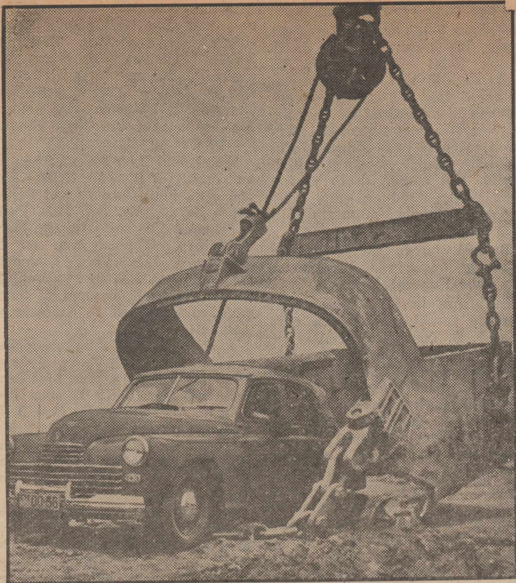
MOUTHFUL —To illustrate the size of the scoop on this electric "walking" excavator—first large mechanical digger in the Soviet Union—a Russian-built "Pobeda" auto is shown being driven into the monster bucket in this picture from an official Soviet source. The giant excavator, put into operation to replace 7000 pick-and-shovel men, according to Russian information, is being used on the construction of the Volga-Don shipping canal.
