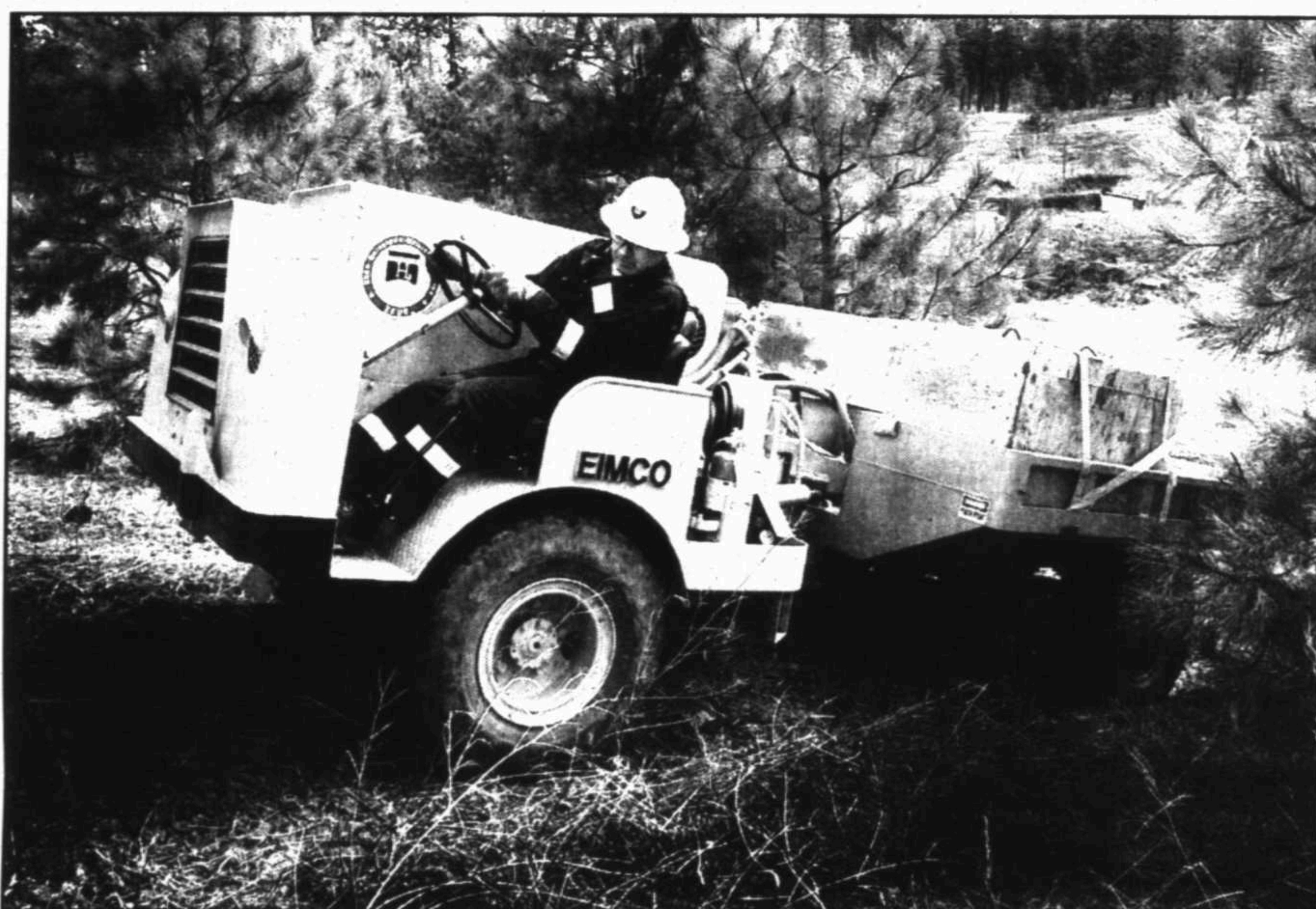
AP Photo Geologist Rich Rains demonstrates a hydrogen powered vehicle for interested spectators from mining and related industries at the Research Labs facility north of Reardan, Wash. The Spokane Research Lab is developing this hydrogen powered vehicle for the mining industry. The lab, intended to make miners safer while assuring a constant supply of strategic minerals, celebrates its golden anniversary this year.
