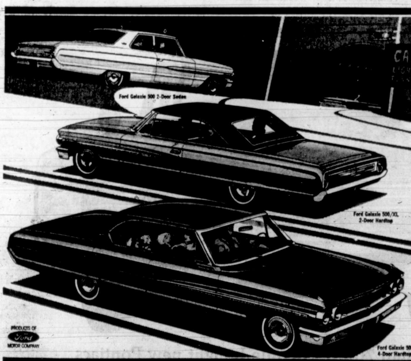
FACTS ON THE 1964 FORD: Choice of three distinctive rooflines • Unique suspension lets wheels move backward as well as up and down to flatten bumps • New comforts and conveniences... more room front and rear with a one-third smaller rear hump... shell-type bucket seats in XL models • Optional Swing-Away steering wheel • Illuminated ignition switch, glove box, ash trays, and trunk in most models • Crank vent windows • Sixteen models • Six engines, from 138 hp to 425 hp • Four transmissions, from America's only fully synchronized 3-speed manual to a 3-speed automatic.
