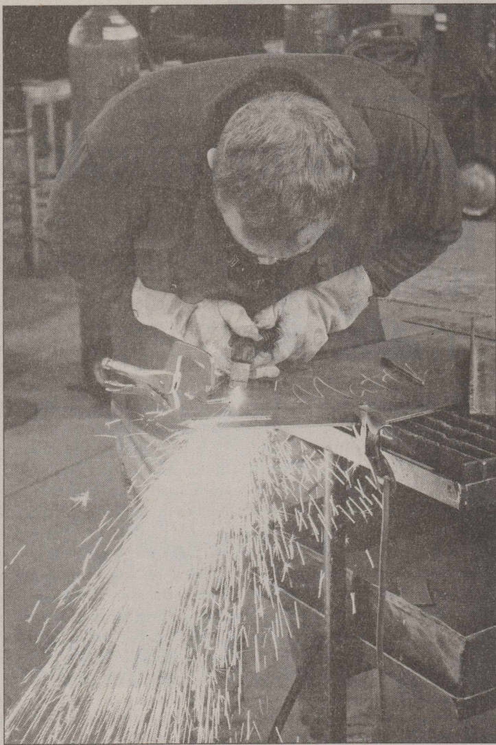
PHOTO BY BRENT SORELLE/The Daily Toreador MATTHEW HUFFMAN, SOPHOMORE agriculture education major from Dallas, uses a plasma cutter on a piece of steel to complete his project in the Agriculture Communication building Wednesday.
