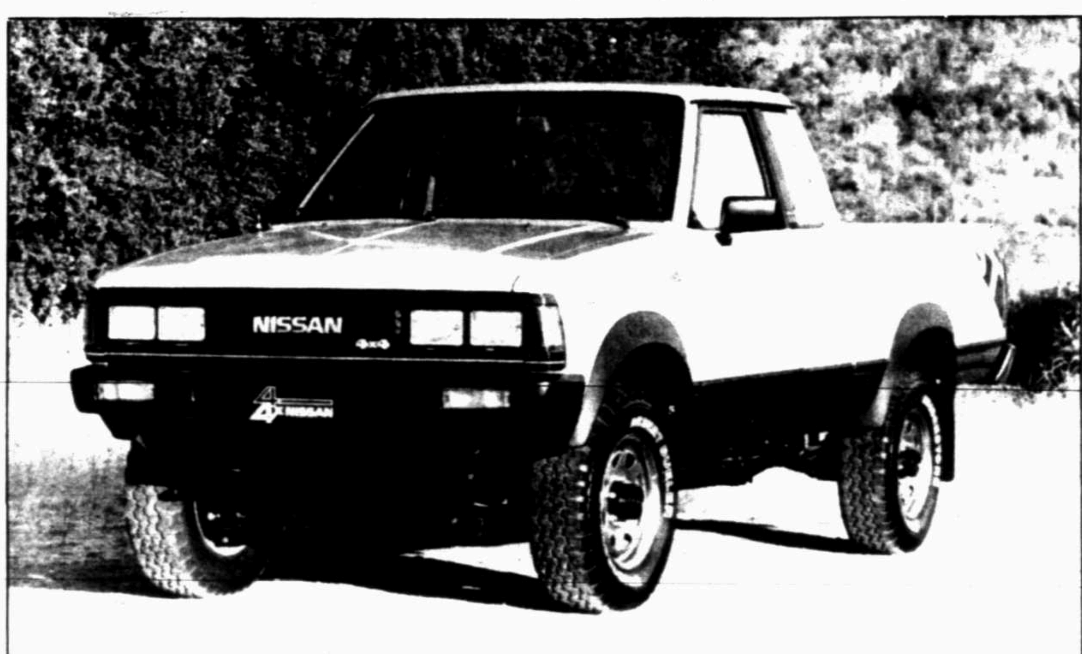
The Nissan 4x4 ST King Cab ST now features increased output along with changes in the gearing and final drive ratio and improved vehicle acceleration.
