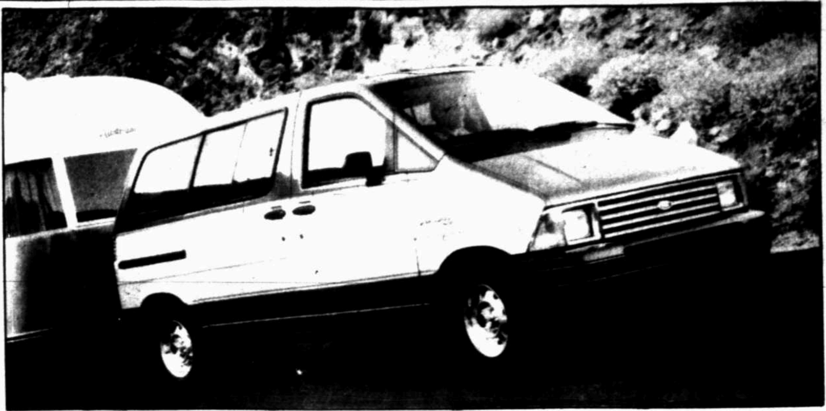
Aerostar's rear-wheel drive and optional 2.8-liter V-6 engine with automatic overdrive transmission have the muscle to tow up to 5,000 pounds
