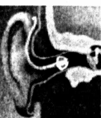
HearStic uses a vented ear bud, which allows natural sounds to pass through without amplification.
