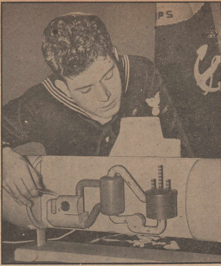
ATOMIC TUMMY—Checking the atomic-engine-filled stomach of this model of the submarine Nautilus, on exhibition at Atlantic City, N. J., is Electrician 1/c, William Christian. The vessel, now under construction at Groton, Conn., will be the world's first atom-powered sub. It will be capable of running for months under water at a speed of 20 knots.
