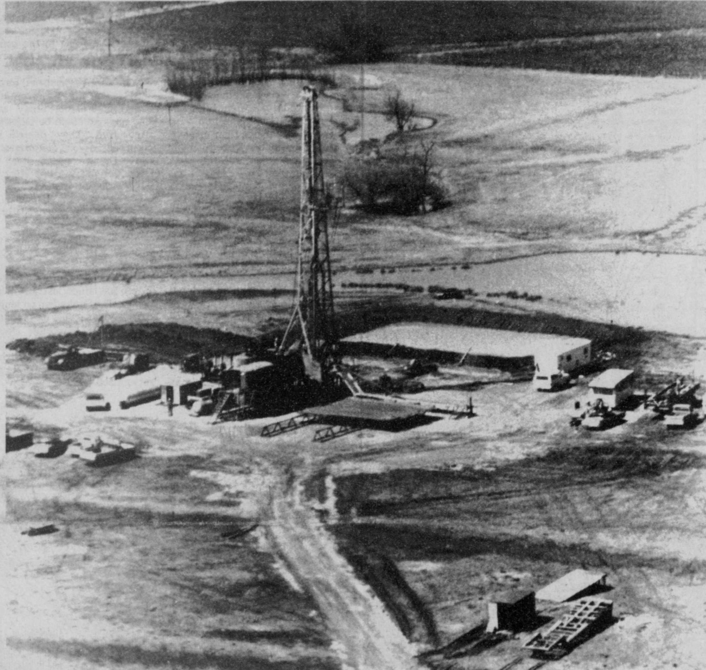
WESTBROOK Drilling Co. is sinking this well for oil and gas on the Dean Ward place near Fulbright. Drilling began March 12, 1978 and will last another 10 days. On Tuesday, the drillers had reached a depth of 3000 feet, with 5800 the maximum. (Staff Aerial Photo)
