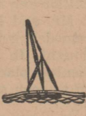
Cranes lifted each new section of pipe to a position on the barges where it could be welded to the section already laid
