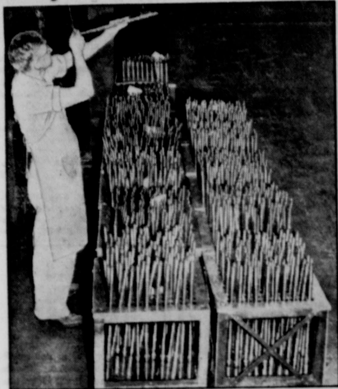
James Halliehan inspects rifle barrels after they have been drilled at Springfield, Mass., arsenal. Plant's commander, Col. G. H. Stewart, has urged War Department to speed expansion to point where output will be 1,000 Garand semi-automatic rifles daily.
