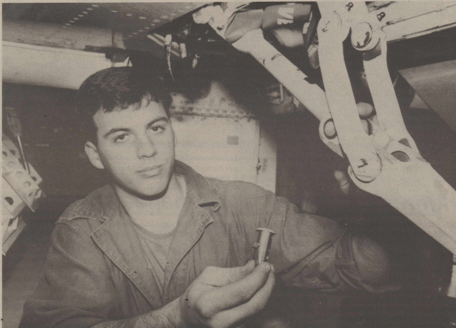
SrA. Sven Christofferson, assigned to the 64th Organizational Maintenance Squadron, Eagle Flight, displays a side brace pivot pin (larger) and bolt from the landing gear. (USAF photo by SrA. Greg Spraggins)
