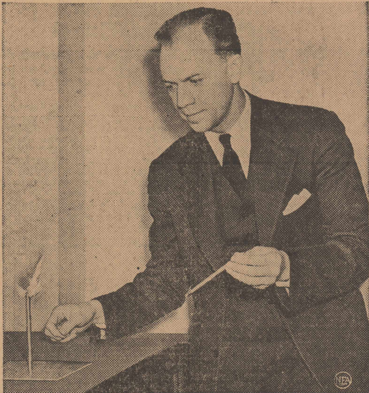
Incendiary pencil, used in cases of sabotage, is presented in flaming demonstration by D. J. Parsons, FBI technician, in New York. Pencil contains ordinary lead and eraser, but also has capsule of acid and incendiary powder. Acid eats through capsule, ignites powder.
