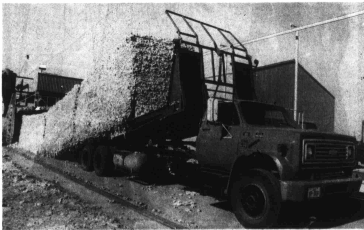
DELIVERING COTTON MODULES TO THE GIN — The module truck picks up the modules from the farmer's fields and transports them to the gin. A module builder builds from 10-11 bales of cotton compressed tightly together.
