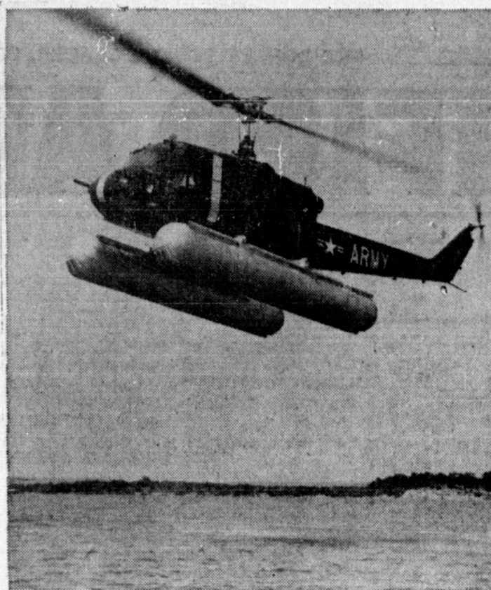
20 YEARS ARMY AVIATION PROGRESS —New application of the Army's versatile IROQUOIS helicopter features amphibious landing gear kit. The kit was developed under a joint Army-Bell Helicopter Co. program and can be used on IROQUOIS HU-1A, HU-1B and HU-1D models. Each air-inflated float bag measures 20 feet long and 33 inches in diameter. The entire unit results in a net weight increase of only 236 pounds. The change from skid landing gear to floats can be accomplished in just 30 minutes by two men.
