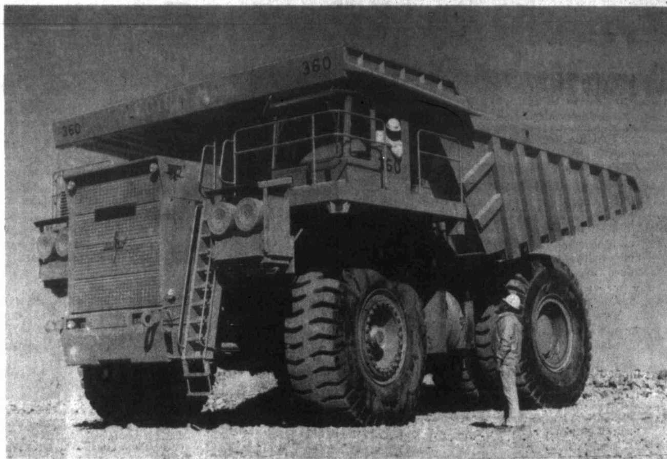
This heavy equipment truck, which operates in the Bingham Copper Mine near Salt Lake City, is capable of hauling 170 tons. It is more than 23 feet wide, 19 feet high and nearly 40 feet long.
