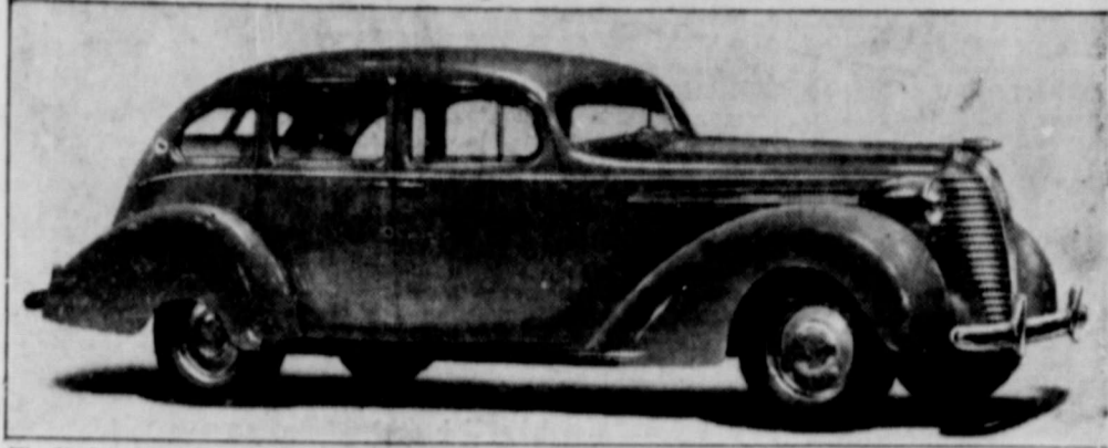
The Hudson Terraplane Sedan in the Deluxe series is on 117-inch wheelbase and has a 96-horsepower engine. The Hudson Super Terraplane, on the same wheelbase, has five additional horsepower.
