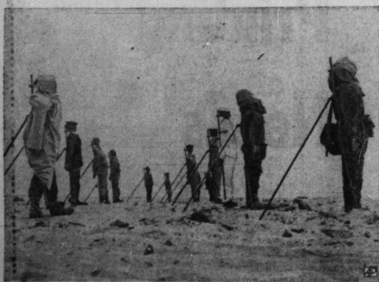
SET UP IN SAHARA —Dummies wearing protective clothing are propped up near the Reggane base in the Sahara Desert for test firing of France's third nuclear device. They were used to determine how troops might survive heat flash and ionizing radiation.
