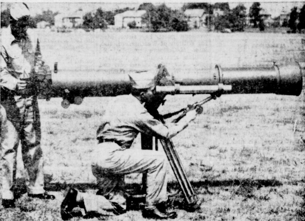
ARMY'S NEW 'BAZOOKA' is not a gun but a camera developed by Army Signal Corps for its new 100-inch infra-red lens. Either this gun-barrel model or the box-type can be carried easily by two men and used five minutes after arrival at the shooting site. The new lens can photograph up to 35 miles away despite fog or haze and substitute for aerial photography when planes are grounded by weather or enemy gunfire. The Army will also use the Peeping Tom lens in television cameras.
